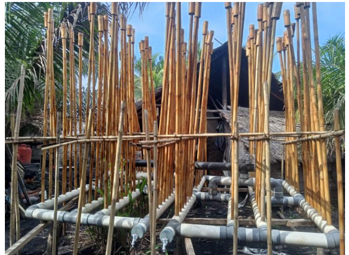
Fig. 1. Placement of thermocouple sensors at the inlet and outlet of the PVC-based smoke condensation pipe within the bamboo-based cooling system.
