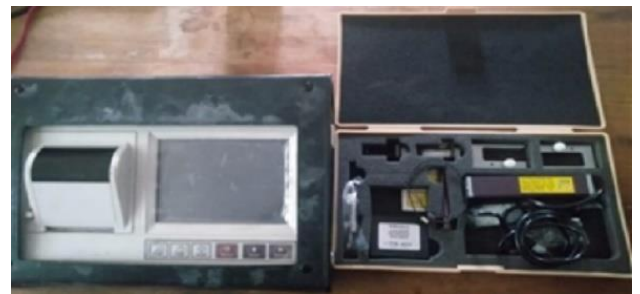
Fig. 4. Mitutoyo SJ-130 surface roughness tester.
