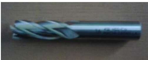
Fig. 2. HSS end mill cutter with 16 mm diameter.
