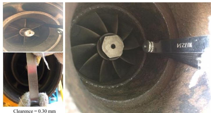
Fig. 4. Result of turbocharger clearance measurement
