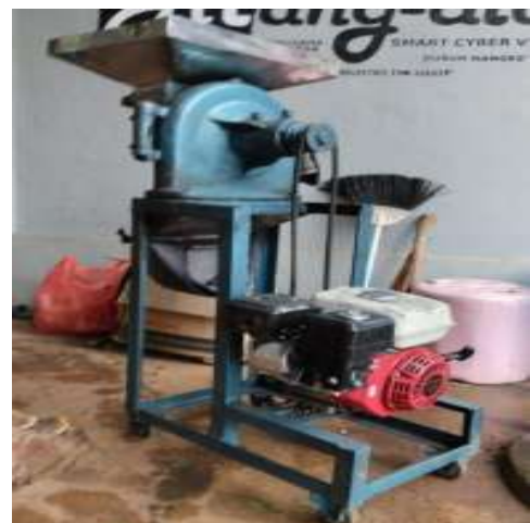
Fig. 1. FFC23 disk mill machine.
