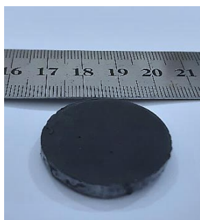
Fig. 2. The dimension of the new MRE sample.
