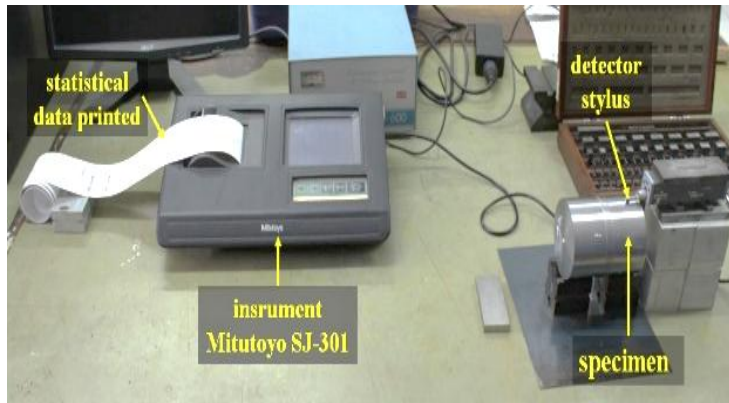
Fig. 3. Surface roughness measurement setup using the Mitutoyo SJ-301 tester.
