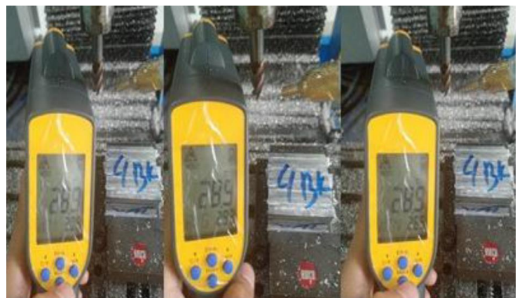
Fig. 7. Machining process temperature measurement.
