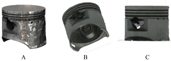
Fig. 11. Images of 3D model texturing object views of different SfM software a. Agisoft Metashape, b. AI Google Colab™, and c. Meshroom
