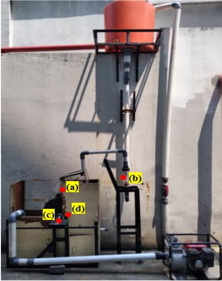
Fig. 5. The assembled overshoot waterwheel installation and data collection location. (a) water flow velocity data, (b) water discharge data, (c) waterwheel torque data, and (d) waterwheel rotation data
