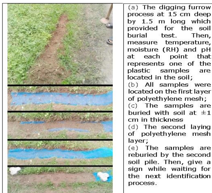
Fig. 17. A situation in the burial process of biodegradable plastic samples in the soil by the first day
