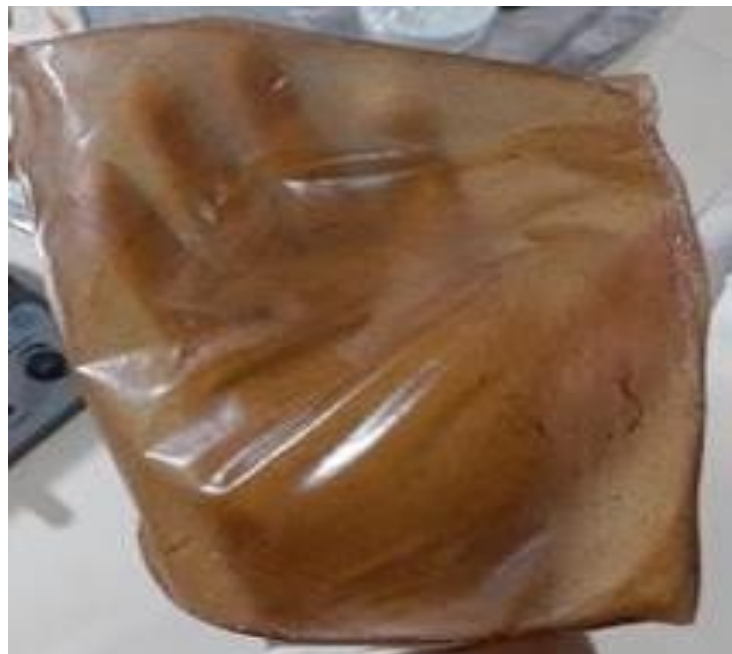
Fig. 3. A physical appearance of mangrove fruit ( Bruguiera gymnorrhiza ) starch-based biodegradable plastic
