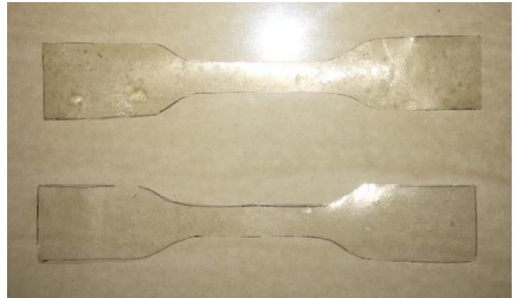
Fig. 7. The manufactured sample for tensile test
