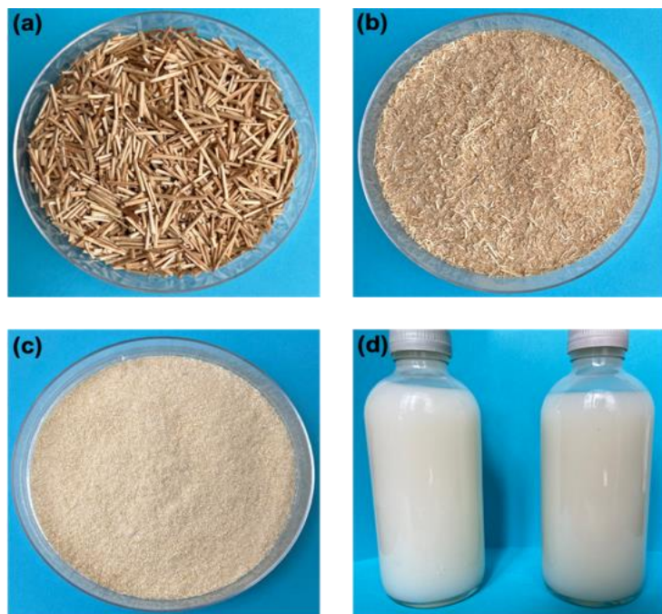
Fig. 2. Visual and structural transformation of OPF fibers after various treatments
