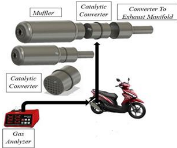
Fig. 1. Exhaust gas emission measurement installation.
