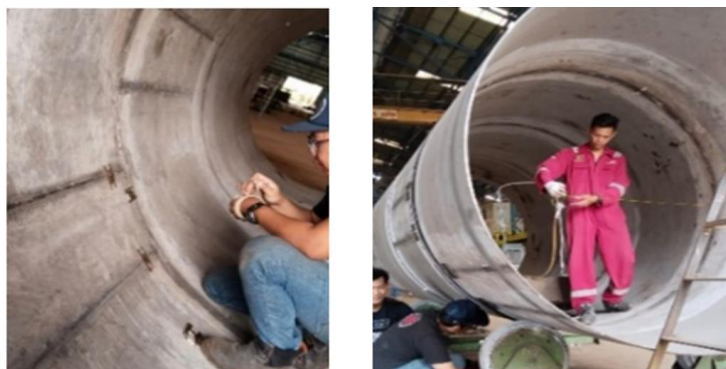
Fig. 2. Film Mounting to Test Object
