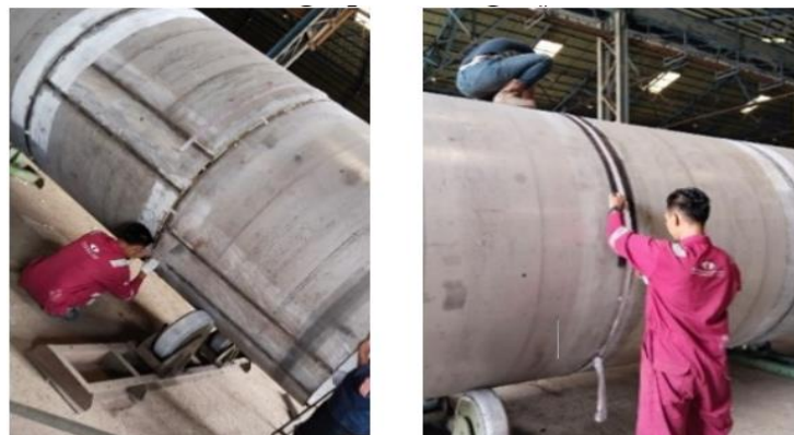
Fig. 1. Radiography Test Shooting Preparation Process
