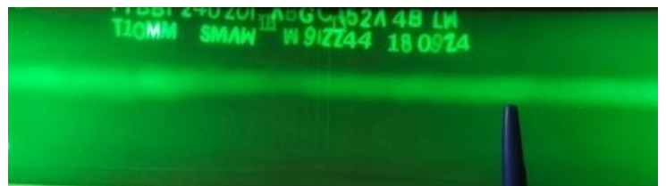
Fig. 6. Film Specimen No. 4-5 Joint No. 1B (LW) (internal source technique)
