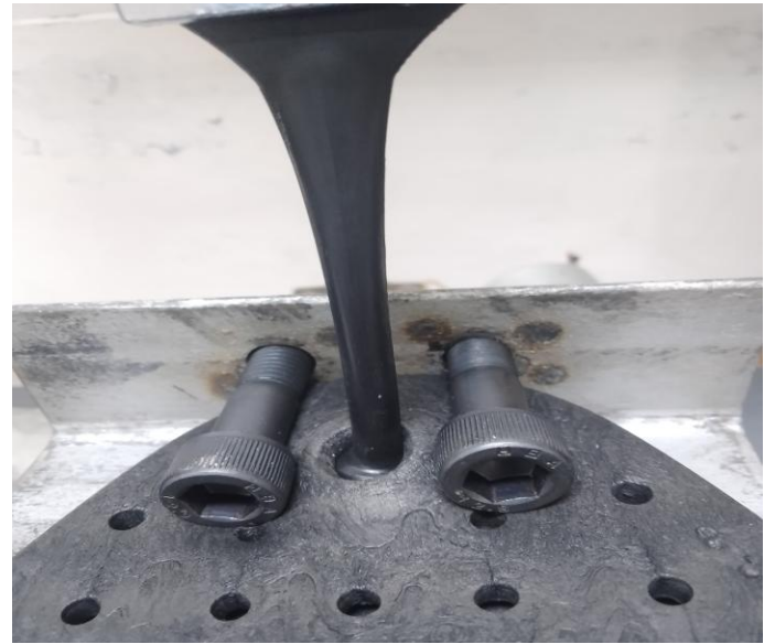
Fig. 5. Tensile force test of the front sandal strap
