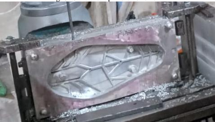
Fig. 4. Sandal base mold for size 41
