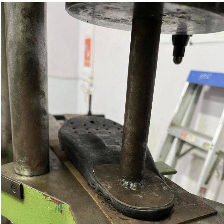
Fig. 8. Compressive test to measure the level of elasticity of the sandal base resulting from injection in the heel area
