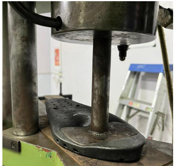
Fig. 9. Compressive test to measure the level of elasticity of the sandal base resulting from injection in the bend area of the foot
