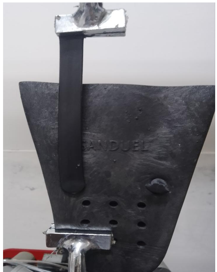
Fig. 6. Tensile force test of left back sandal strap
