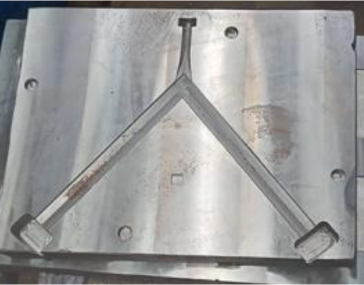
Fig. 3. Sandal strap mold for size 41
