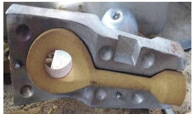
Fig. 3. The RCS core on the aluminum mold
