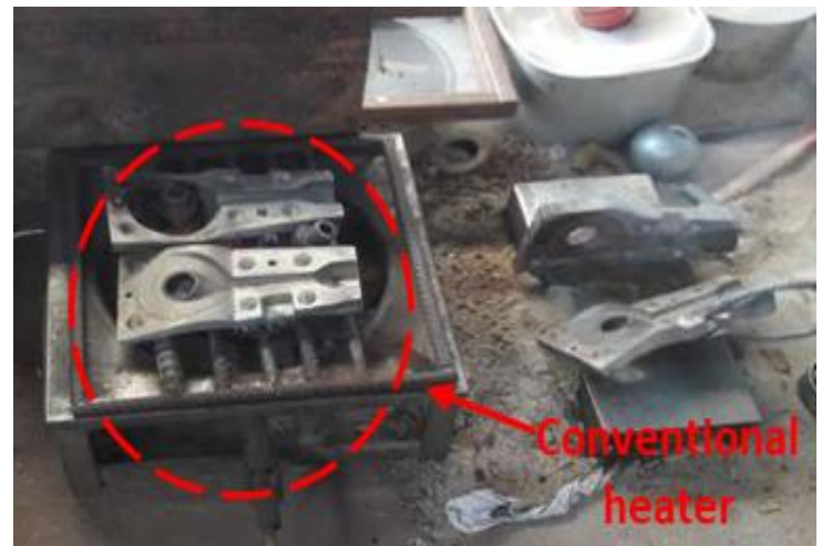
Fig. 2. Heating the aluminum mold using a conventional heater
