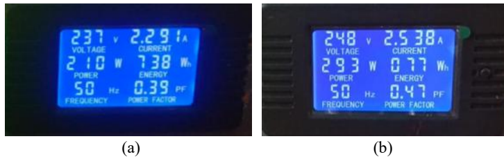
Fig. 15. Digital power meter measurement in: (a) automatic mode; and (b) manual mode
