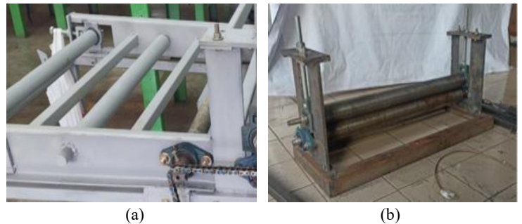
Fig. 3. (a) Conveyor frame; and (b) roller
