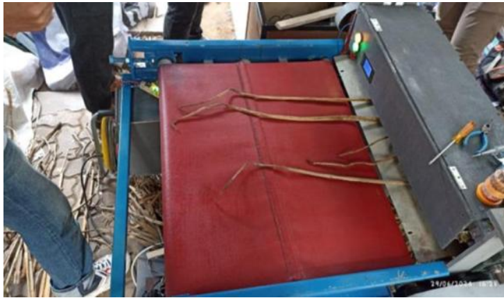
Fig. 10. Automatic flattening machine testing for flattening 5 common water hyacinths
