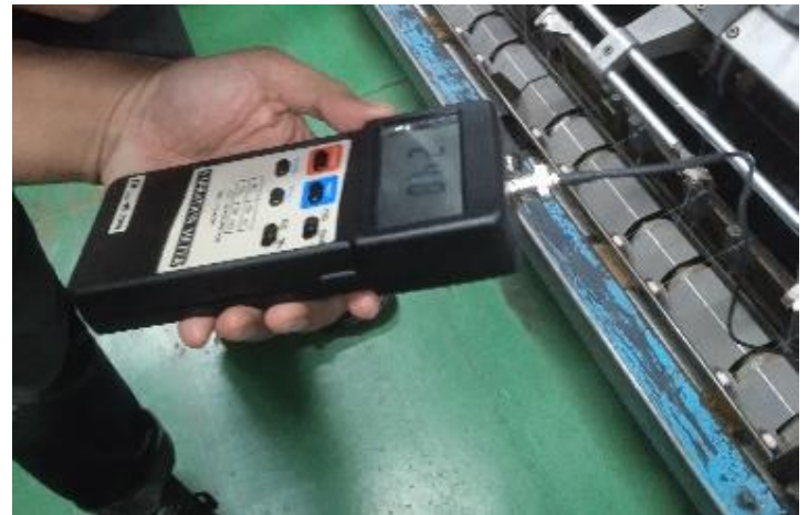
Fig. 7. Calibration process using Lutron VB-8200 Vibration Meter.
