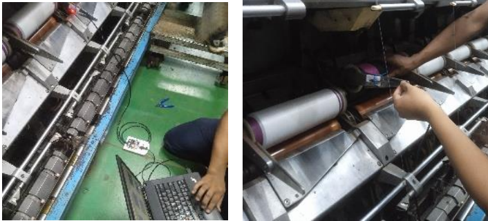
Fig. 9. Sensor mounting position on spindle arm.
