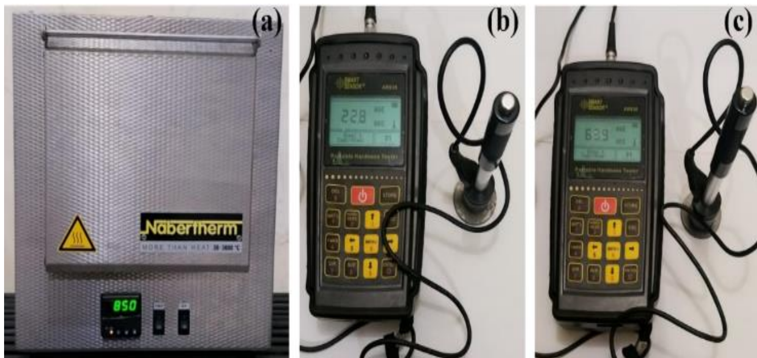
Fig. 2. Material Preparation of SKD11: (a) heat treatment process (JIS G 4404 standards), (b) hardness measurement prior to heat treatment, and (c) hardness measurement after heat treatment.
