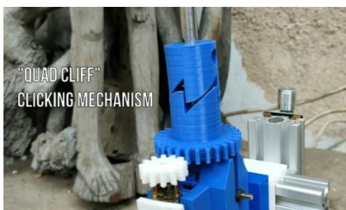
Fig. 5. Quad cliff clicking mechanism.
