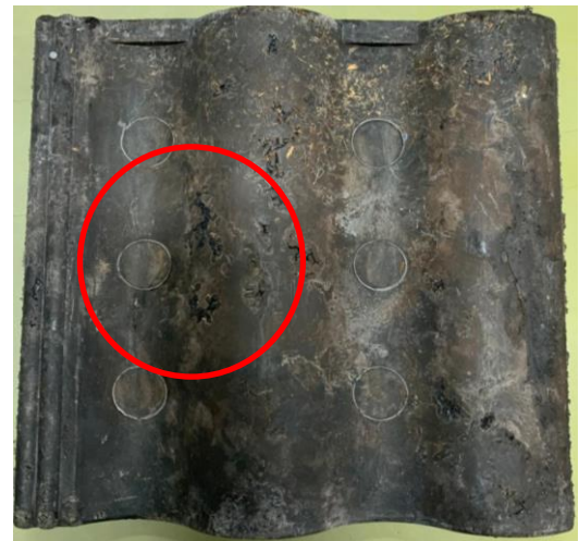
Fig. 9. Product results with uneven heating.
