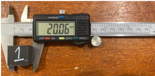
Fig. 5. Dimensional measurements on test specimens.
