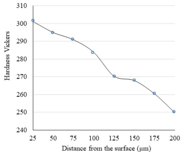
Fig. 4. Cross-section hardness of the combined carburizing and shot peening specimen surface.
