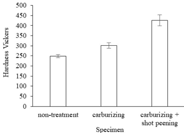
Fig. 3. Surface hardness graph of non-treated, carburized, combined carburizing, and shot peening gear-sprocket specimen.
