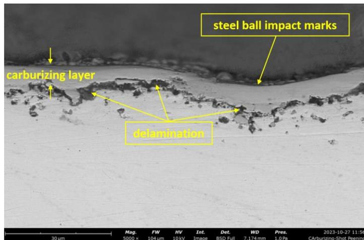
Fig. 5. Cross-section microstructure of combined carburizing and shot peening specimen.
