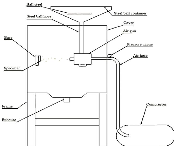
Fig. 2. Schematic diagram of shot peening process.
