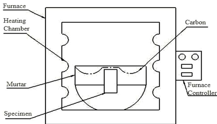
Fig. 1. Schematic diagram of the carburizing process.
