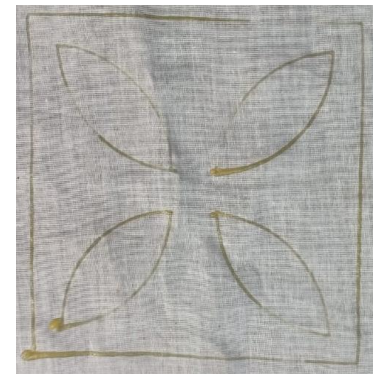
Fig. 5. The results of the canting pattern at a temperature of wax 70 °C with feed rate 300 mm/ min
