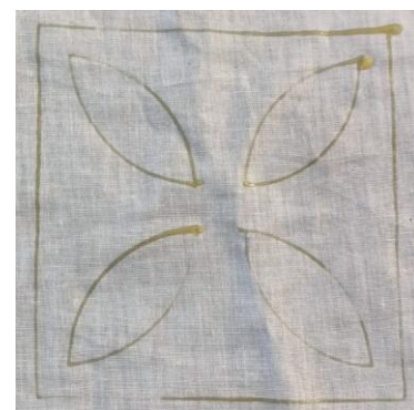
Fig. 6. The result of the penetration canting pattern at temperature wax 70 °C with feed rate 300 mm/ min
