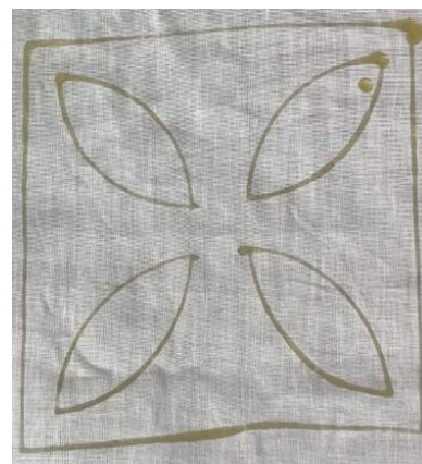
Fig. 9. The results of the canting pattern at a temperature of wax 90 °C with feed rate 450 mm/ min
