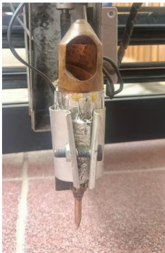
Fig. 3. Electric canting with 1mm nozzle
