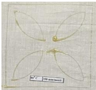
Fig. 7. The results of the canting pattern at a temperature of wax 80 °C with feed rate 350 mm/ min
