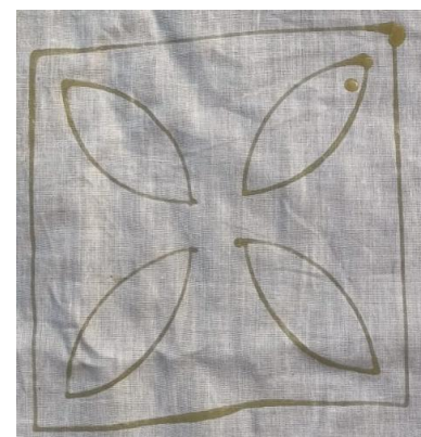
Fig. 10. The result of the penetration canting pattern at temperature wax 90 °C with a feed rate 450 mm/ min
