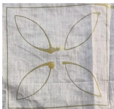
Fig. 8. The result of the penetration canting pattern at temperature wax 80 °C with feed rate 350 mm/ min
