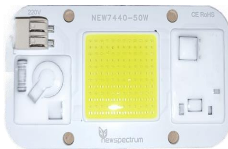
Fig. 2. The chosen high-power LED lamp for wide-area illumination.
