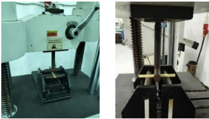
(a) (b) Fig. 9. Composite bending testing.
