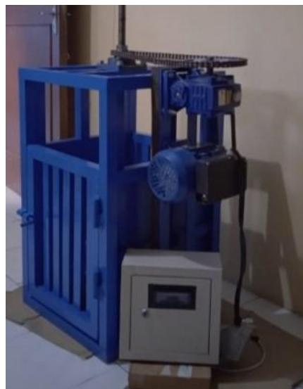
Fig. 2. Can pressing machine by utilizing lead screw and a microcontroller-based monitoring system.
