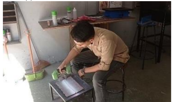
(b) Photo testing specimens with magnetic particles (PT)
