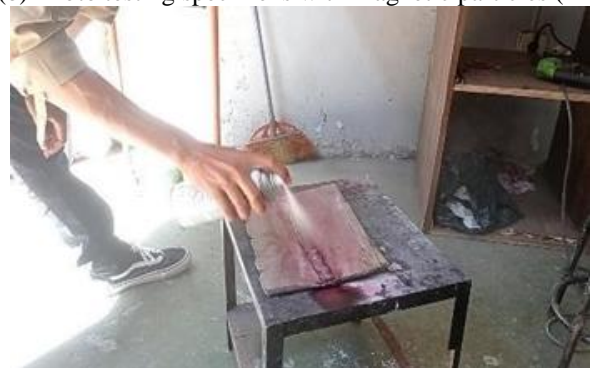
(c) Photo testing specimens with Penetrant Test (PT)
