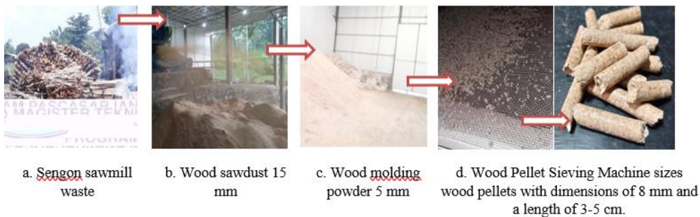
Fig. 2. Process material into wood pellet.
