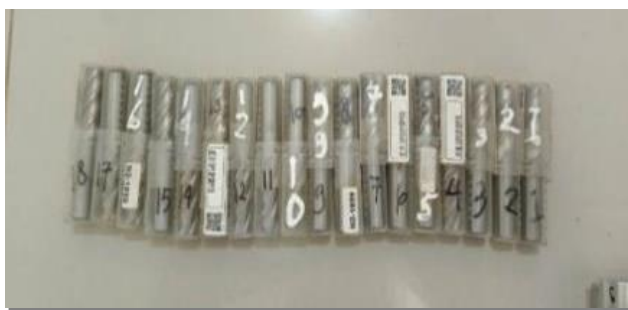
Fig. 1. Endmill HSS (10 mm 4 flute).
