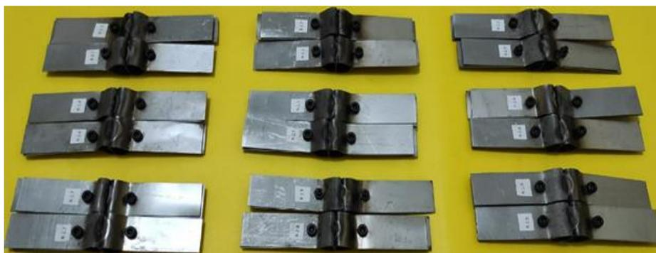
Fig. 5. 18-unit sample TIG welding using different thickness low carbon steel.
