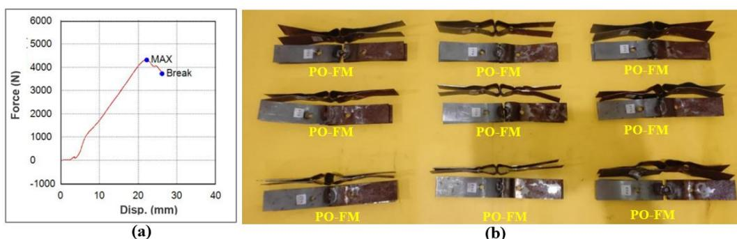
Fig. 6. The load of TIG welding. (a) The highest DT-load chart as recommended by the Taguchi experiment, and (b) pull-out failure mode.
