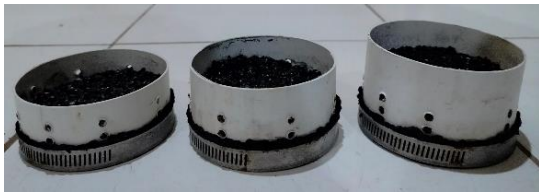
Fig. 2. Charcoal processing: charcoal after being mashed is put in a tube.
