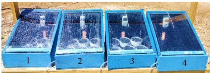
Fig. 5. The fogging process on the glass surfaces of basins 1, 2, 3 and 4 at 9:30.
