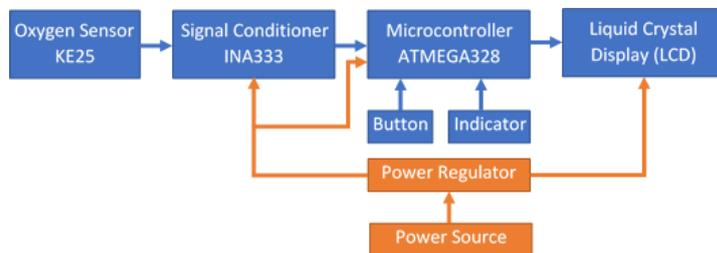
Fig. 3. Design diagram of the oxygen concentration measuring instrument.
