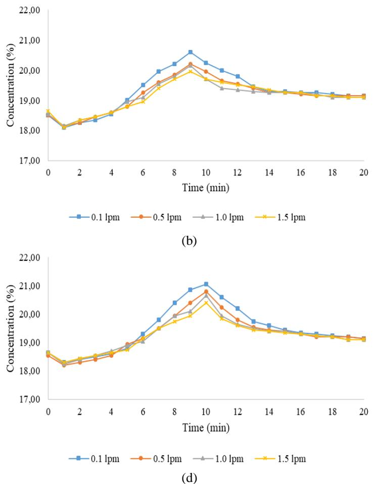
Fig. 5. Oxygen concentration in the PSA process with various zeolite activation temperature variations (a) 250°C (b) 300°C (c) 350°C (d) 400°C.
