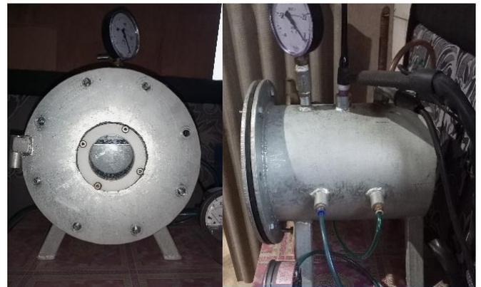
Fig. 1. Vacuum chamber with a glass observation window.
