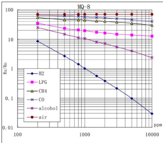
Fig. 5. The MQ 8 sensor gas characteristic curve.
