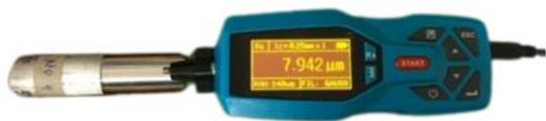
Fig. 1. Surface roughness tester MR-220.
