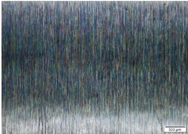
a) Surface roughness 6.445 \mu\text{m}
