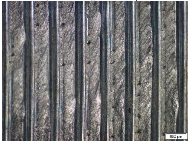
b) Surface roughness 21.280 \mu\text{m}
