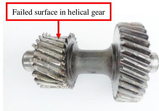
Fig. 1. Helical gear failure.
