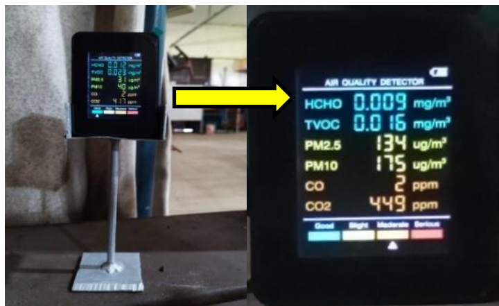
Fig. 8. Tools for measuring chemical elements in welding operations.
