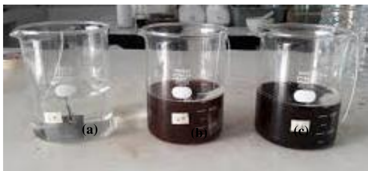
Fig. 2. Preparation of solution: (a) 3.5% NaCl solution, (b) temiki extract, (c) rubek's extract.
