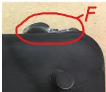
Fig. 6. Flashing defect products[23].
