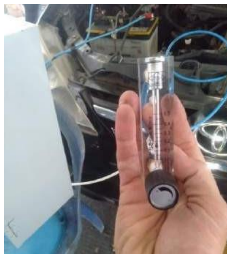
Fig. 3. The appearance of brown gas production in the flow meter.
