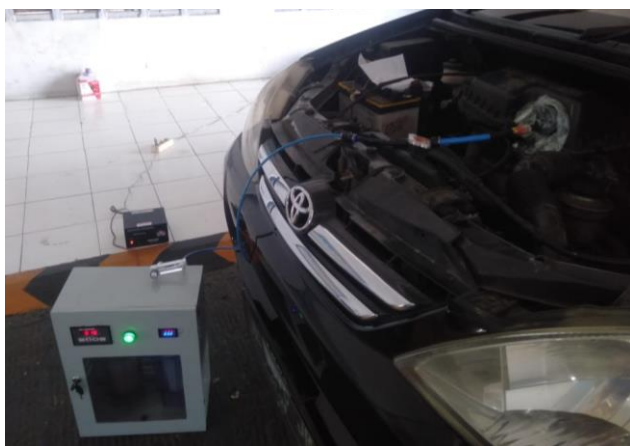
Fig. 4. The process of introducing brown gas into the incoming air flow of gasoline engine.
