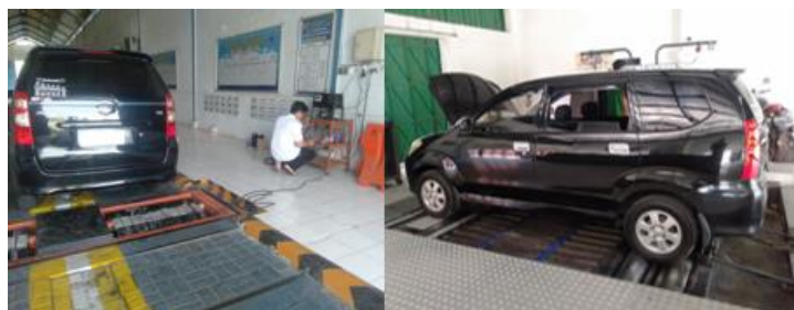
Fig. 5. The process of collecting power and emission test data.
