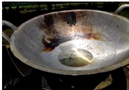
Fig 7. Illustration of the experiment involving the heating of coconut oil using a solar cooker equipped with chrome sticker reflectors.
