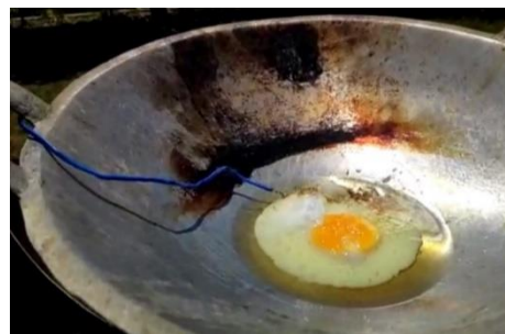
Fig8. The experiment involved frying an egg using a solar cooker equipped with chrome sticker reflectors.
