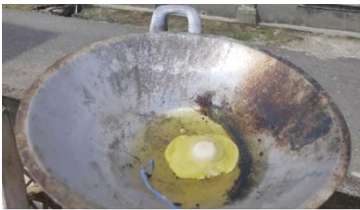
Fig 10. Illustration of the experiment involving egg frying using a solar cooker equipped with a glass mirror reflector.
