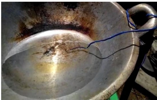
Fig 6. Experiment with boiling water using reflectors made from chrome stickers.
