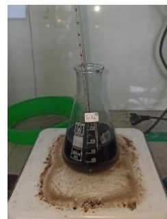
Fig. 4. Washing of crude bio diesel.
