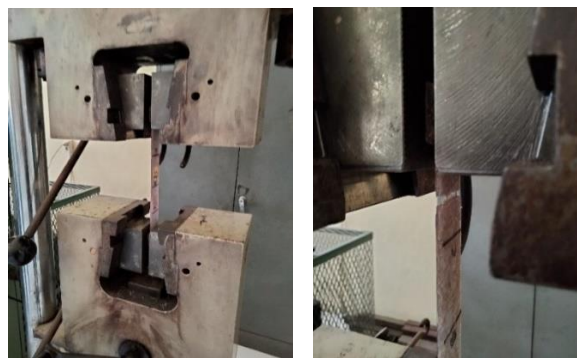
Fig 9. Tensile testing is carried out to obtain tensile strength, which is by distributing the tensile force with the material area unit using Eq. 1 [44], wher \sigma is Stress or stress (MPa), P is Tensile Force(N), and A is Cross-sectional Area (length x width) mm 2 .
