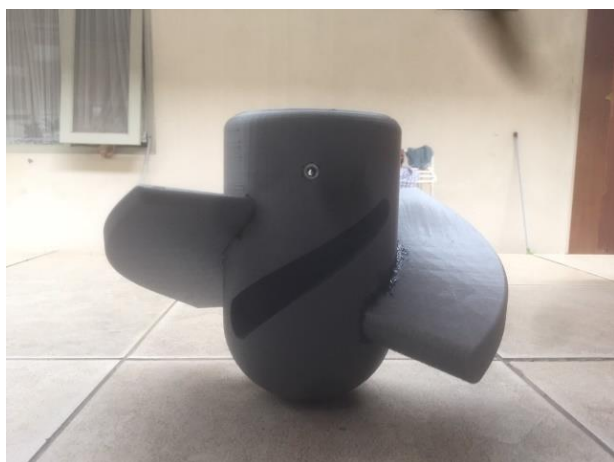
Fig. 12. Assembly turbine with runner.
