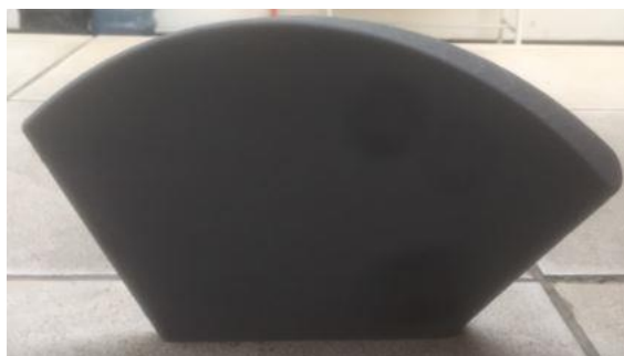
Fig. 13. 3D print of guide vane.
