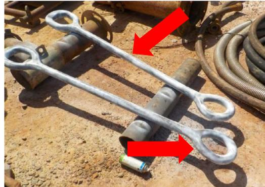
Fig. 7. Elevator link inspection.
