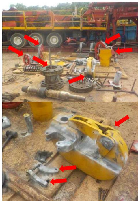
Fig. 2. Traveling block and hook block magnetic particle inspection.
