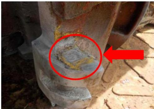
Fig. 6. Crack on pin lock tubing elevator door 2-7/8".
