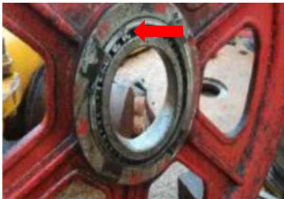
Fig. 3. Crown block visual inspection.
