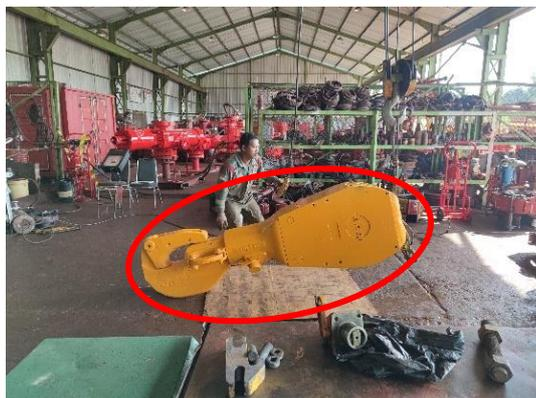
Fig. 1. Traveling block and hook block visual inspection.
