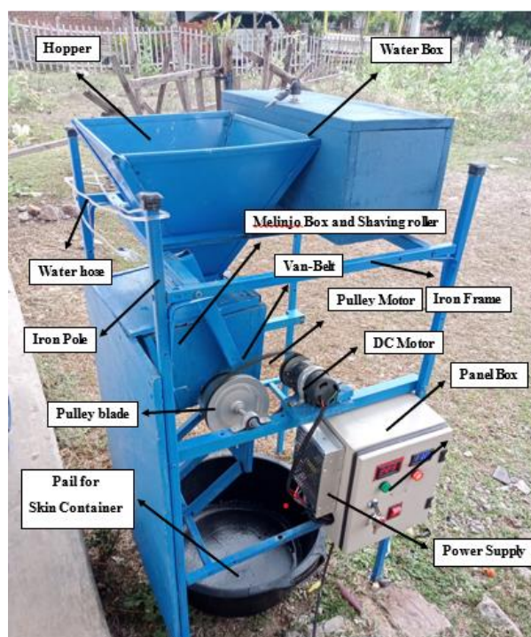
Fig. 8. The realization of the melinjo fruit outer skin peeler prototype design using a grate roller based on auto-reverse movement control built upon Fig. 6.
