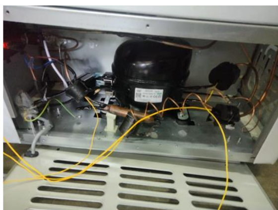
Fig. 2. Thermocouples to measure compressor suction and discharge temperatures as well as condenser temperature.
