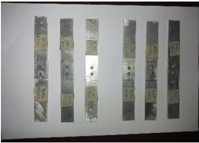
Fig. 20. Results of installing the drill and FSW methods.
