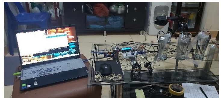
Fig. 4. Experimental set-up for testing the thermal performance of stainless-steel ice cubes.
