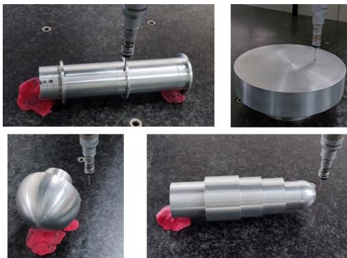
Fig. 13. The measuring process of the workpiece specimen using the CMM.
