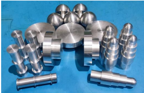
Fig. 12. Specimens of the cutting test result.
